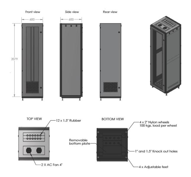
Meet to with standard ANIS/EIA-310D-1992 (Rev.EIA-310-C), IEC 60297-1, IEC 60297-2, BS 5954:Part 2, DIN 41494. ETS 300 119 Manufacturing standard ISO 9001: 2000 Company.
